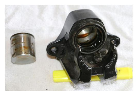
The Piston may be slightly pitted from rust and this is okay, as long as the pits do not run vertically up the side and as long as there aren't too many.
