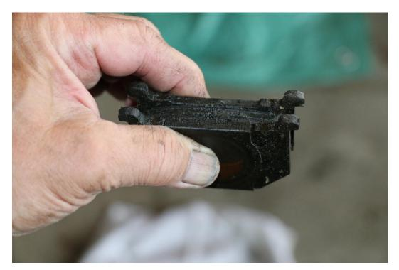
The Pad Guides should be shiny clean. The pads slide along these guides so it is essential they are clean. In this caliper they were coated with brake dust and dirt and had to be removed with a pick, after removing some of the crud. There is one on each side.
