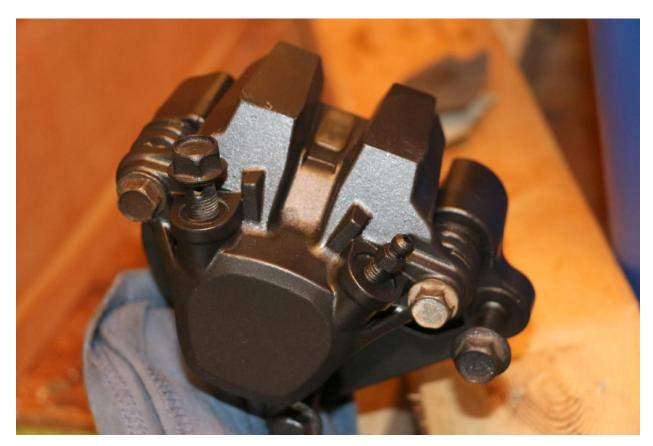
If the axles spin while tightening the bolts they are flattened so you can grasp them with pliers. Once the bolts are tight, you should be able to move them in and out so they settle into place.
