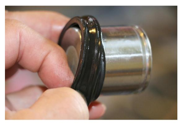
Once it is started I find it easiest to use a clamp and gently and slowly ease the piston into the bore. It will hesitate slightly at the Seal but should slip past it.
