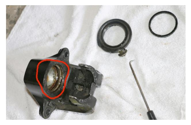
Now comes the most time consuming part – cleaning the bore. You can see the attached "stuff" on this bore. And you can see some of the corrosion in the grooves for the Boot and the Seal.
