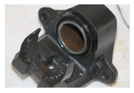
Now you can take this assembly and re-install the Pad Spring. It fits so the rectangular cut out is exactly over the Sight Hole. The tangs should slide down into the sight hole and may or may not hold it in place. You may have to hold it while placing the Caliper Body onto the Caliper Holder.
