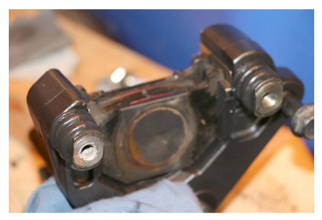
To reassemble the Caliper body the first step is to lightly coat the inside of the bore with Brake Fluid.
