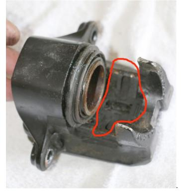
Next, you can tackle the Caliper Axles. They are different in that one of them has a sleeve on it. If the calipers are extremely dirty, or have been sitting for a long time, the one with the sleeve can be difficult to remove and may have to be pulled with pliers. The sleeved axle is always the one farthest away from the bolts that hold the caliper to the fork.
